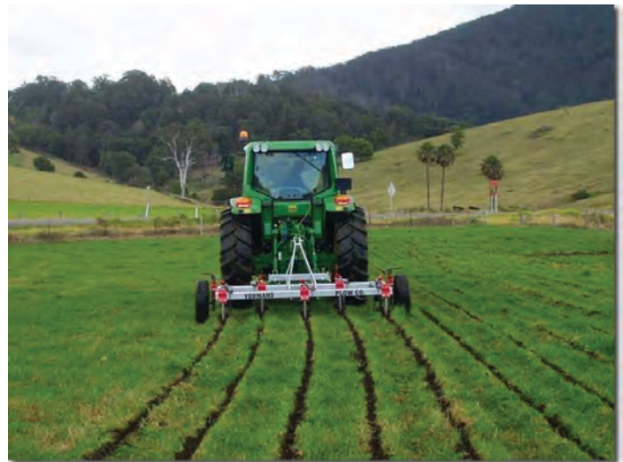
The Yeomans or keyline plow. Photo from Permaculture Research Institute ( https://www.permaculturenews.org/2014/07/30/tera-tracked-earth-repair-apparatus-for-large-scale-earth-repair/ )
